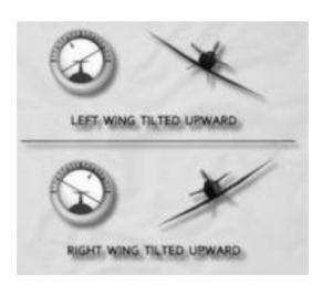
To answer the questions, you will have to use information from both the compass and artificial horizon to determine how the plane is oriented. If the plane is flying north, it will appear to fly into the page in the illustrations.
